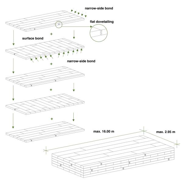
Each layer is micro planed, glued then pressed in a hydraulic press until cured.
